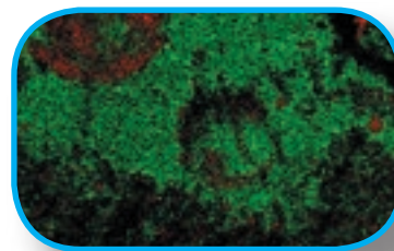
X-ray microanalysis overlay of the same specimen is used to further differentiate oil from water content (green: oxygen, red: carbon)
