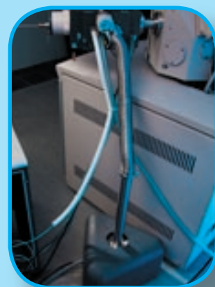
Off-column turbo-pumping system
