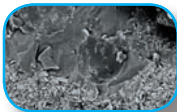
Oils and rocks. Chalk rock saturated with brine and oil. Dark grey bubbles are oil droplets in brine-filled cracks
