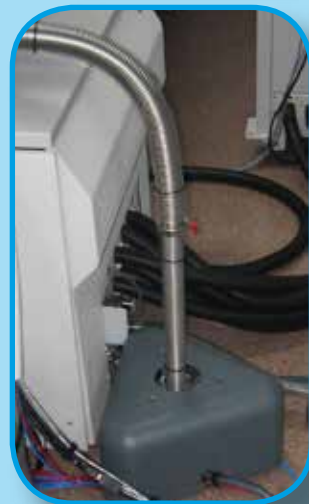
Off-column turbo-pumping system
