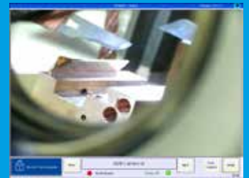
Images of both specimen cold stages can be expanded to fill the whole screen. Video images can be captured and saved
