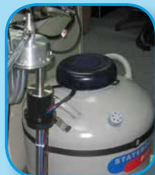
Off-column cooling system with up to 24 hour runtime
