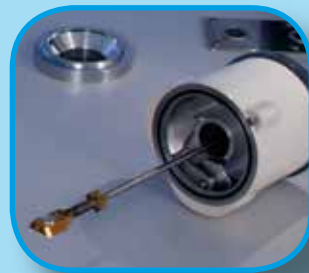
Cryo transfer device with specimen shuttle and stub insert
